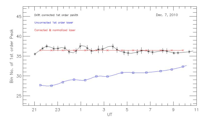
Our ideal data taking scheme is to take laser calibration exposures throughout the night, interspersed after two cycles of N, S, E, W, zenith mirror pointing cycles on the sky. These laser calibrations allow us to track any spectral drift that may occur in the instrument during a night, and thus permit the extraction of vertical winds relative to a nightly average.
