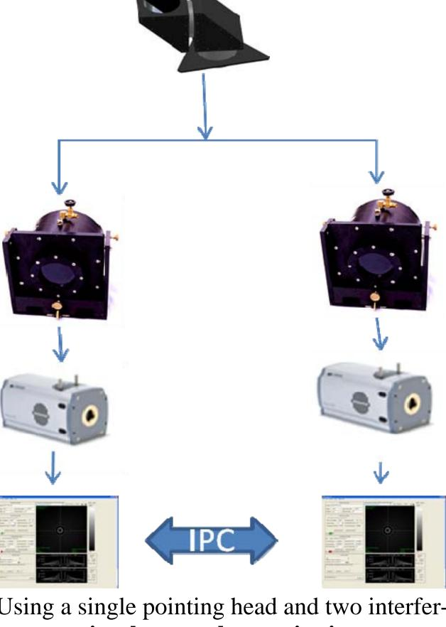
ometers simultaneously acquire images at different wavelengths. Synchronized acquisition realized through inter-process communi cation between multiple instances of Image-Tool on the network.
